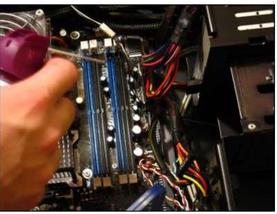
If you've got a fan that's particular gunked up, don't be afraid to use a cotton swab with a bit of isopropyl alcohol to get the blades clean. Give the fans a quick spin to make sure that the blades move freely after cleaning. If they don't, it's probably best to go ahead and replace those fans. You can buy these from Jaycar.
