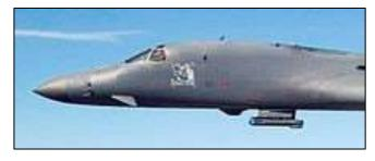
and fixed intake ramps, which limit its speed compared to the B-1A. Vanes in the intake ducts serve to deflect and shield radar emissions from the highly reflective engine compressor blades. The B-1A's engine was modified slightly to produce the GE F101-102 for the B-1B, with an emphasis on durability, and increased efficiency. The nose gear cover door has controls for he
