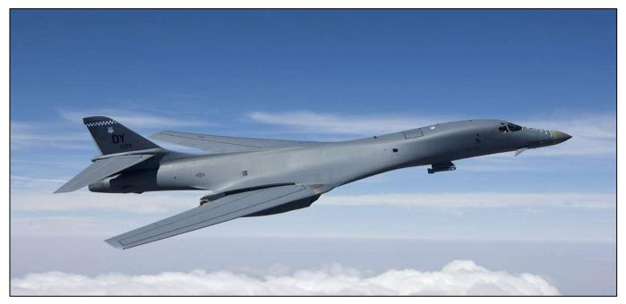
The B-1B's maximum take-off weight was increased to 216,000 kg from the B-1A's 179,000 kg. The weight increase was to allow for take-off with a full internal fuel load and for external weapons to be carried. Rockwell engineers were able to reinforce critical areas and lighten non-critical areas of the airframe, so the increase in empty weight was minimal. To deal with the introduction of the MiG-31 equipped with the new Zaslon radar system, and other aircraft with look-down
