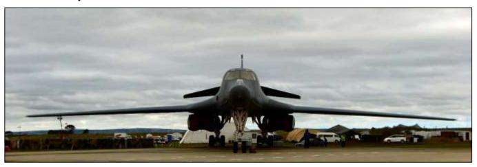
The B-1, which was built by Rockwell International (now part of Boeing) is a supersonic variable-sweep wing, heavy bomber. It is commonly called the "Bone" (from "B-One") and is one of three strategic bombers in the U.S. Air Force fleet, the other two being the <u>B-2 Spirit</u> and the B-52 Stratofortress.
