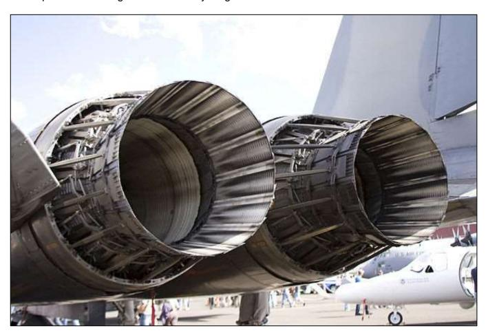
In order to achieve the required Mach 2 performance at high altitudes the exhaust nozzles and air intake ramps were variable. Initially, it had been expected that a Mach 1.2 performance could be achieved at low altitude, which required that titanium be used in critical areas in the fuselage
