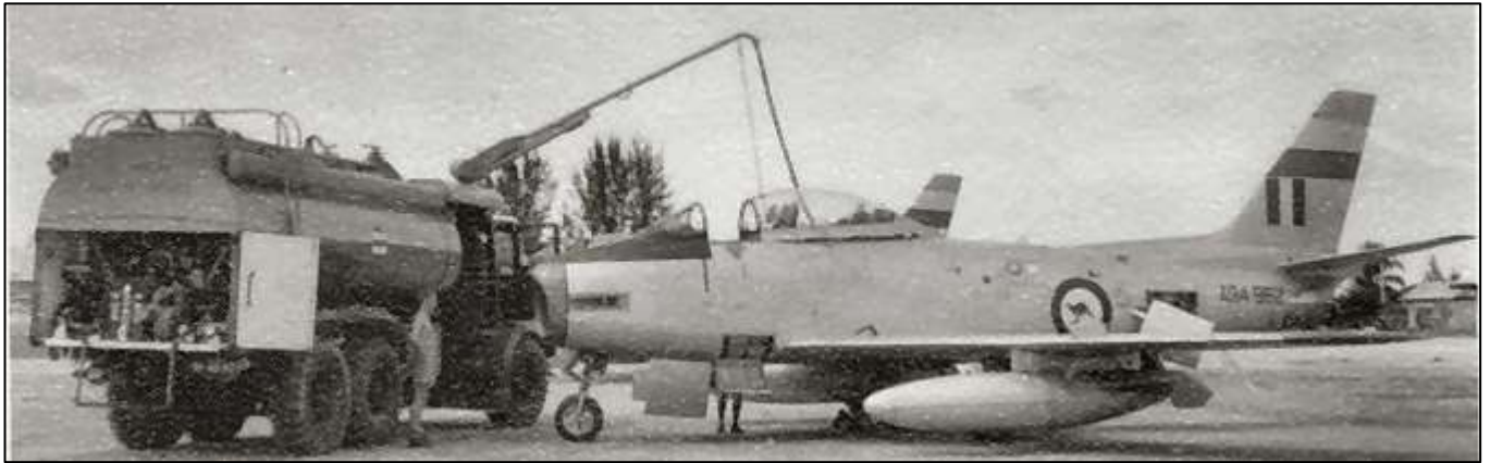
A Labuan fuel truck tops up the starboard "jug" of A94-962
