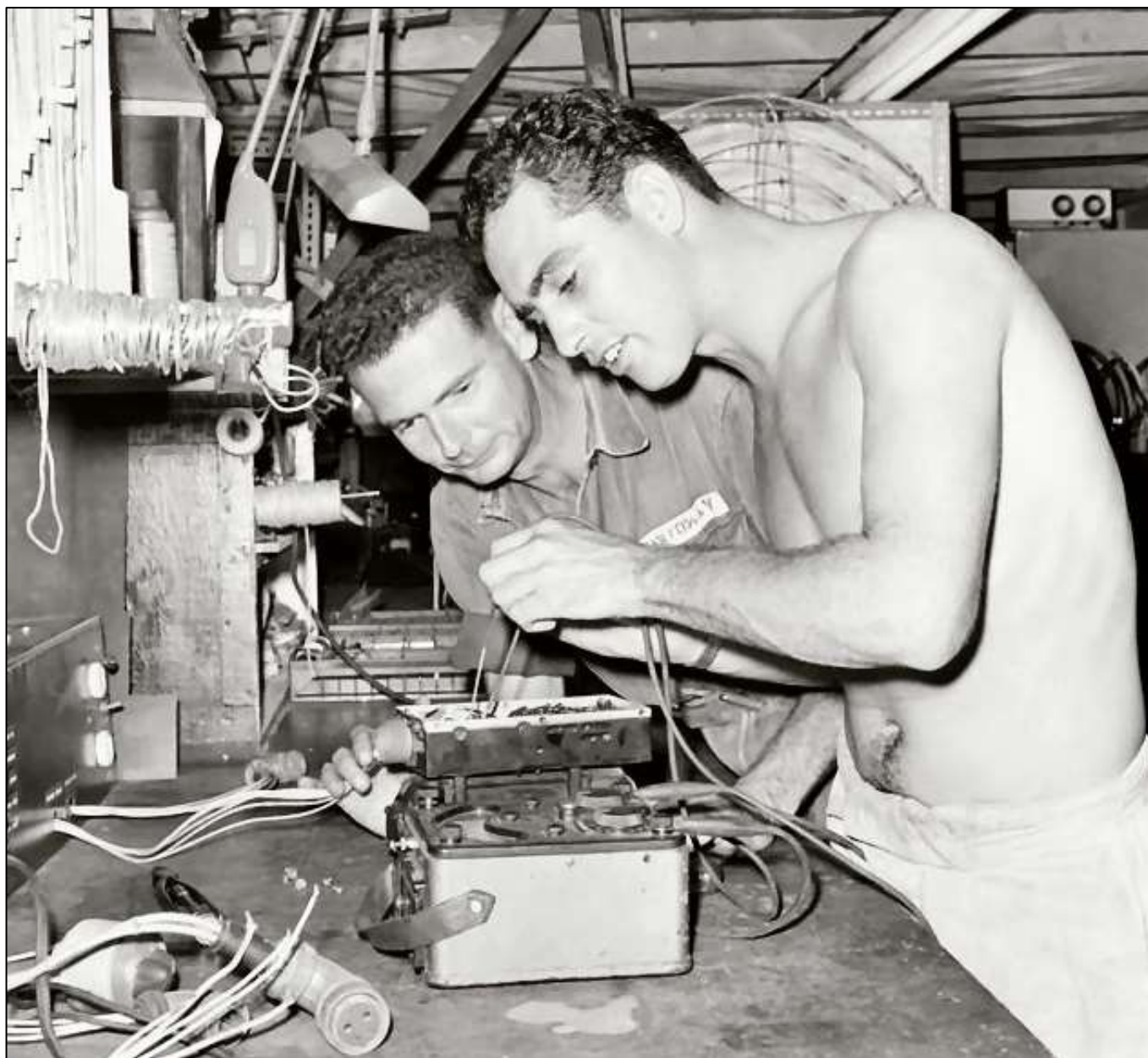
Electrical fitter Tom Van Dyken (left) supervises Ray "Luigi" Hanlon who is testing a Caribou aircraft's inverter which supplies AV power to various instruments. March 1966.
