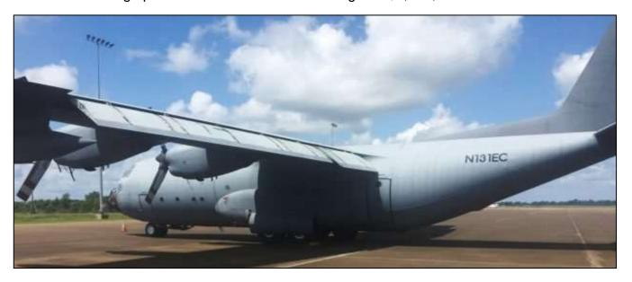
First flown in 1954, the C-130 proved to be highly manoeuvrable and its pressurized hold accommodates troops or cargo, both of which can be dropped into battle. The high-wing design and integral rear ramp eases loading and unloading. Popular Mechanics called the C-130
