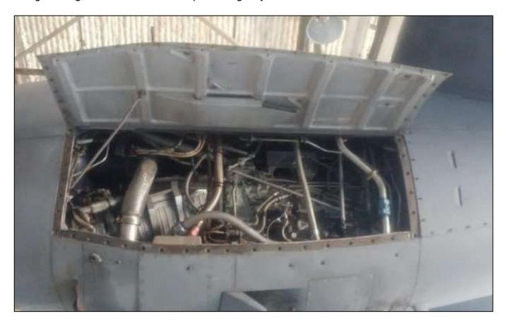
The Herc is normally driven by four Allison T56-A-IA turboprop engines which produce 3,750 HP each but only two engines are described in the listing which could be a problem as the A model is a lot happier with four. Like many wedding singers, the Curtiss-Wright propellers feature variable pitch.
