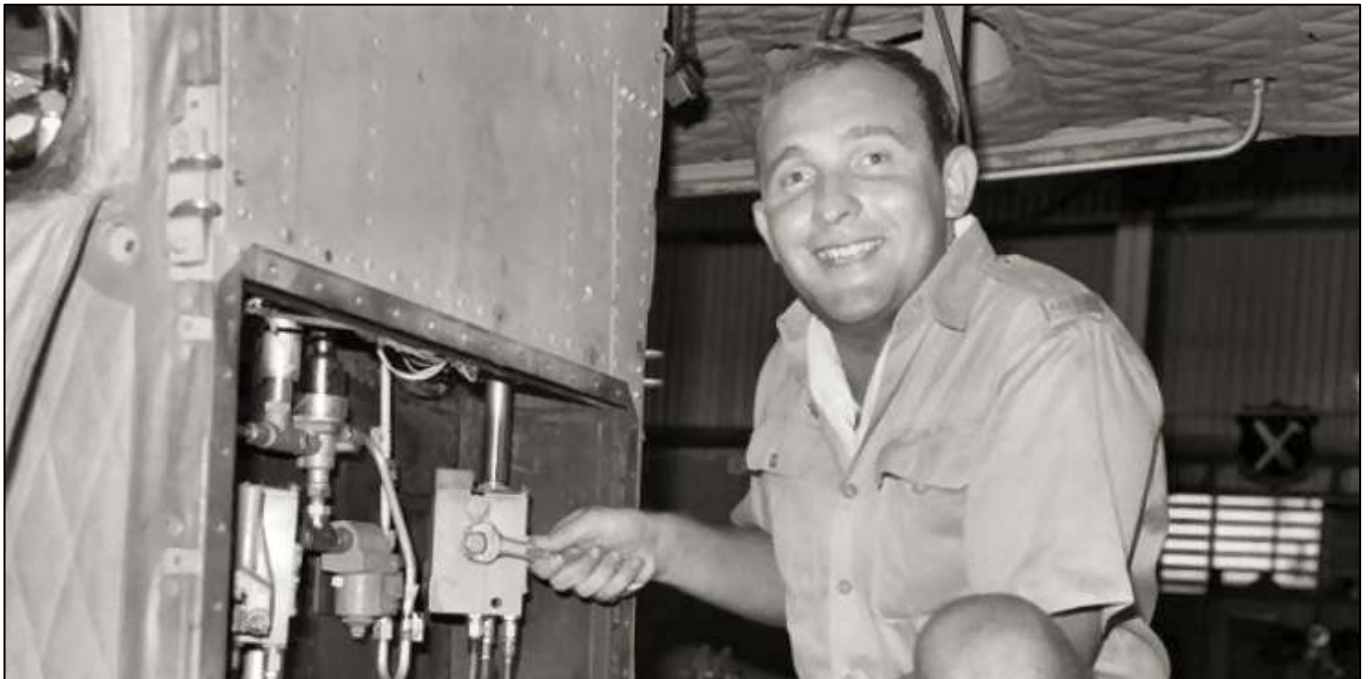
Peter Tickner, 9 Squadron, (Framie) is checking the hydraulic union on an Iroquois. June 1969.
