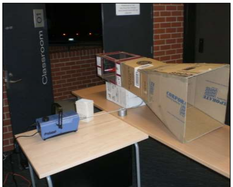
The 315SQN AAFC Wind Tunnel set up with a smoke generator.
