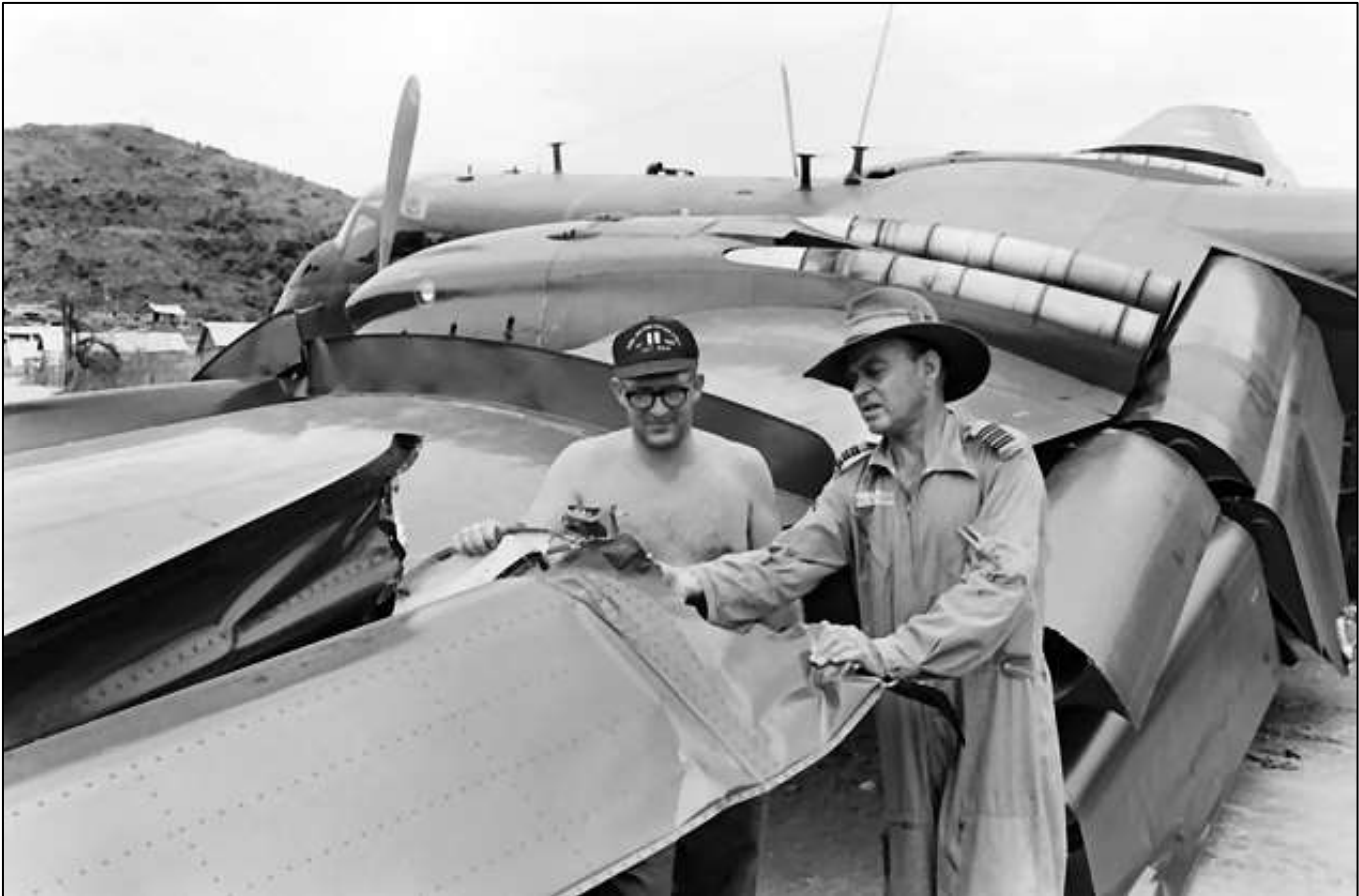
35 Squadron, Engineering Officer, Herbert (Wally) Solomons, and the CO Charles Melchert, inspecting the crashed Caribou for the extent of damage and to make a list of the parts required to make it airworthy.
