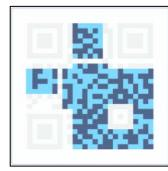
The error correction mechanism inherent in the QR Code structure is where all data vour is contained, also sharing the space with the error correction blocks that allow up to 30% of the Code to be damaged.
