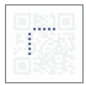
Alternating black/white modules on the QR Code with the idea of accurately helping configure the data grid. Using these lines, the scanner determines how large the data matrix is.
