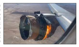
Such an event is extremely rare and happens when huge spinning discs inside the engine suffer some sort of failure and breach the armoured casing around the engine that is designed to contain the damage.
