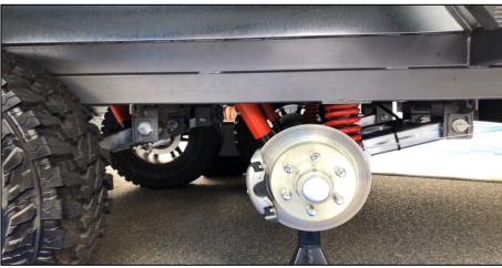
definitely a better brake in pure stopping power. Importantly, discs are less prone to brake fade in the way that a drum might on long downhill sections or arduous conditions.
