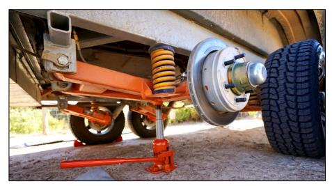
over-ride or electric, and anything over 2000kg needs brakes on each wheel, which is usually electrically operated drums but occasionally more complex hydraulic/air disc brake systems.
