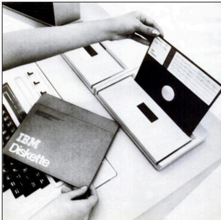
*The IBM 3740 Data Entry System marked the first appearance of the “IBM Diskette.”*
