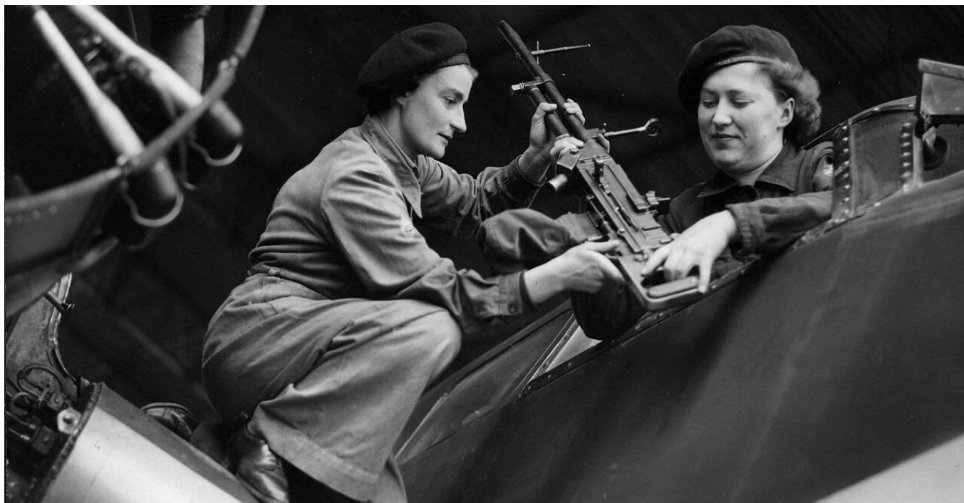
WAAAF armorers, Margaret Deal and Rosemary Kemp, installing a Vickers machine gun into an aircraft.
