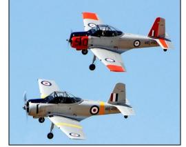
The Winjeel was a three seater with two front seats with dual controls and a third seat rear. The Pratt & Whitney R-
