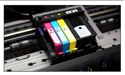
The next step is releasing ink droplets through these nozzles at a very precise rate. Manufacturers delicately engineer the ink in terms of viscosity and pigment density to ensure that it's always the same amount of ink and that it looks just right on the page. For colour printers, there are often hundreds of separate nozzles for the different colour inks, in addition to the ones for the black ink.
